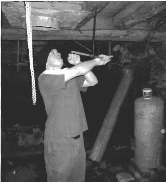
Fig. 3 Sampling of the basement beams in the structure. Note the bark still visible on most of the beams.
